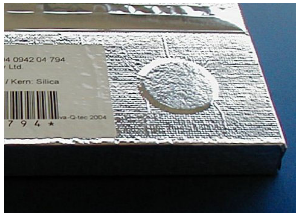
Fig. 5: Metal sensor chip integrated into a vacuum insulation panel
