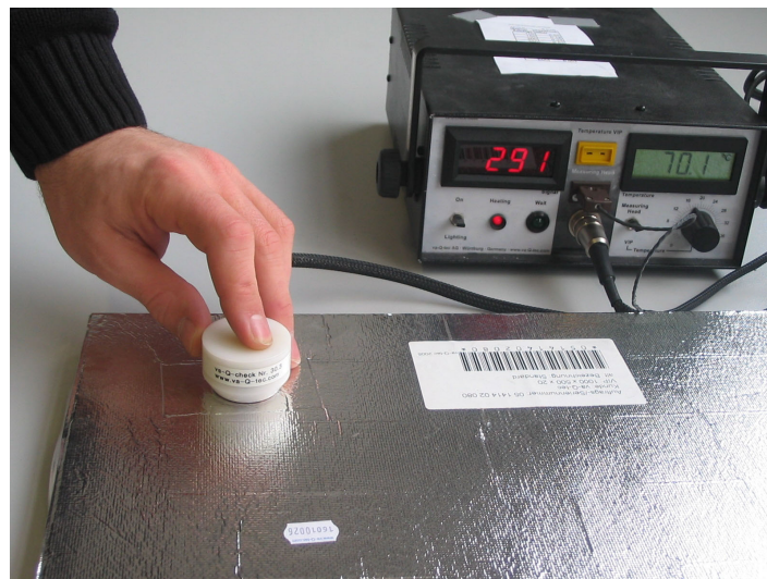
Fig. 6: Measurement of gas pressure with “va-Q-check”
